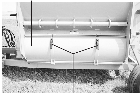
clean out door latches
