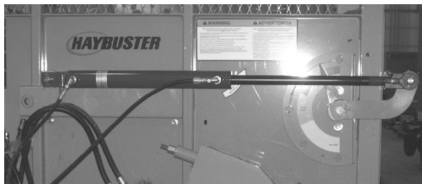
Hydraulic slug bar cylinder shown in the highest raised position
