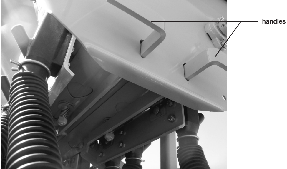
drill cleanout slides
