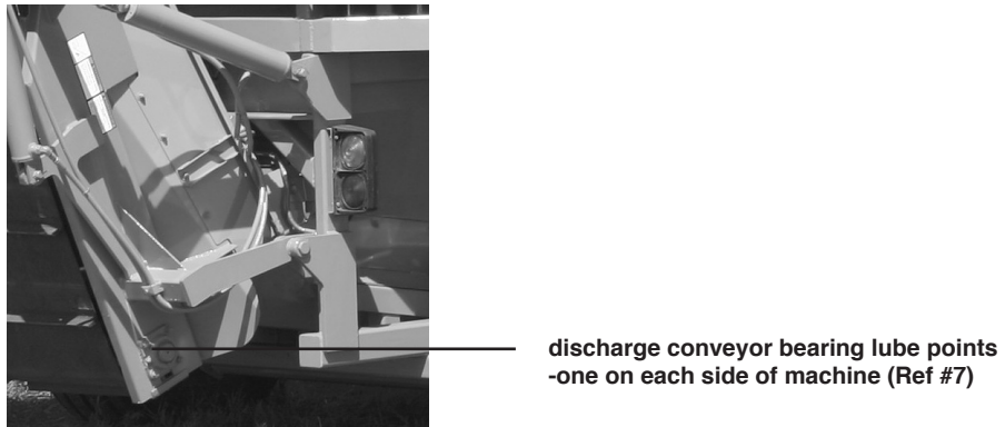
Figure 3.9 discharge conveyor bearings lubrication points (2 of 4)
