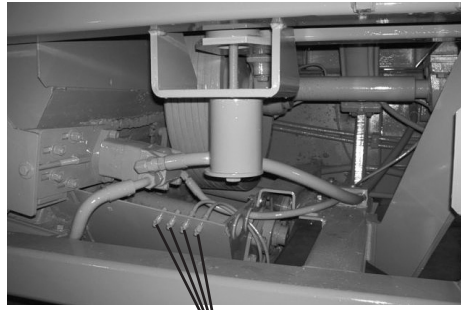
belly auger bearing lubrication points (Ref #5)
