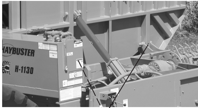
tub pivot lubrication points (Ref #4)
