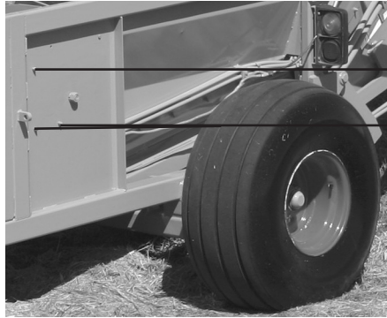
front rotor bearing lubrication points 1 of 2 (Ref # 3)
