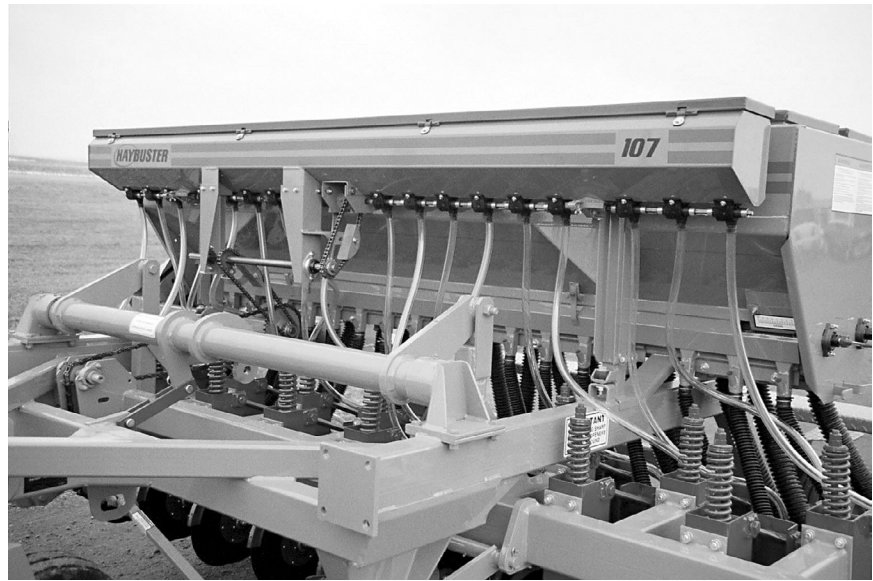
Cover and above photo show the legume box installed with optional drop tube assembly
